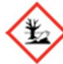
Environmental Impact Hazard
